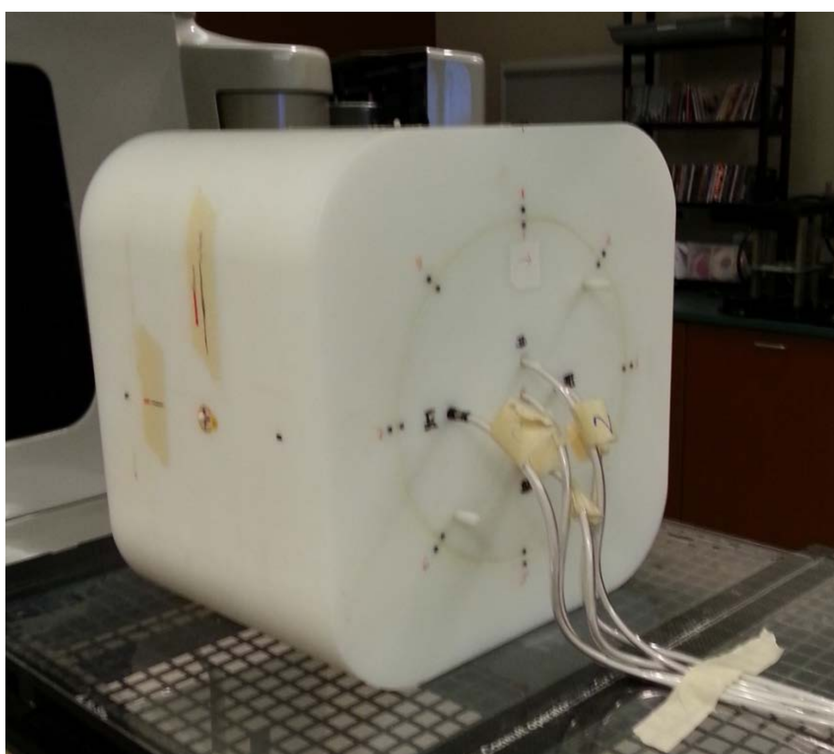
Figure 1: Multiple ion chamber phantom used as gold standard for classifying acceptable and unacceptable plans
